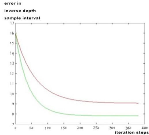
Fig.5 Overall error of depth estimation comparison within 380 iteration, green:cost column fixing, red:anisotropic regularization term
