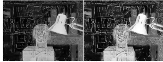
Fig.4 Recovered depth map. Left: cost column fixing; Right: anisotropic regularization
