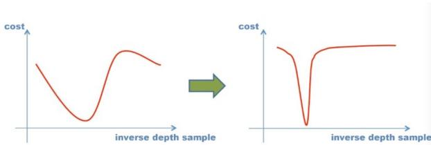
Fig.3 Idea of fixing the confident feature point depth. Left: original  $C_r(d)$ . Right:  $C_r(d)$  with given minimal.
