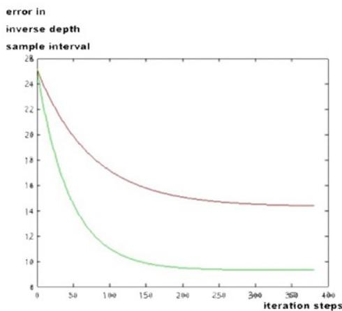
Fig.6 Plot of average error of depth estimation for selected highly textured smooth area within 380 iteration, green: cost column fixing, red: anisotropic regularization term
